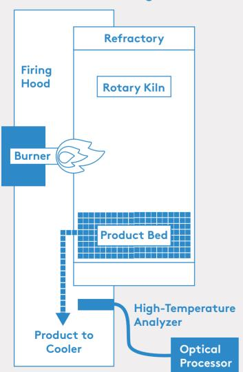
The Blue Cube High Temperature Analyzer probe is mounted below the kiln, viewing particles falling to the discharge chute or product cooler.
